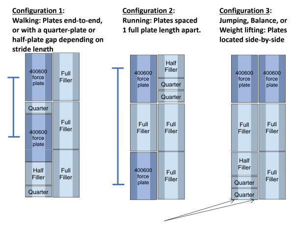
Mounting rail pair (shown behind). Each pair is the length of one force plate.
