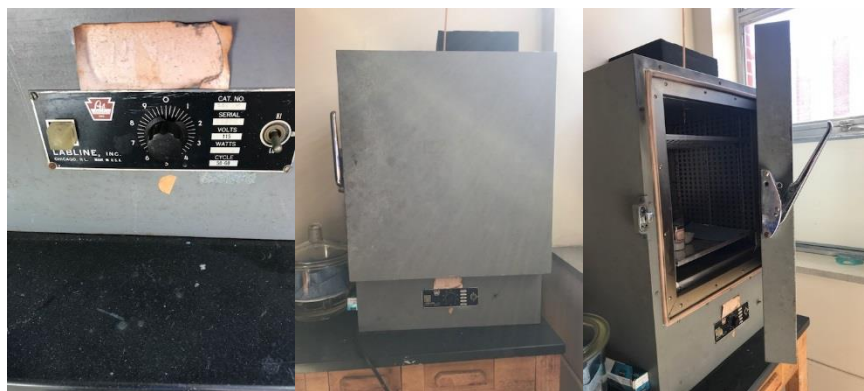
Images: front control panel of oven (left), oven (center) and broken latch of oven (right)
